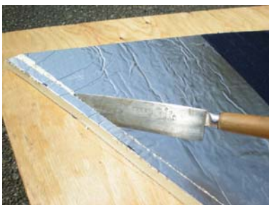
Figure 2: freehand angular cut
